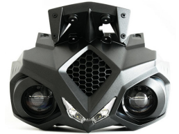
Energica Eva electric motorbike 3D printed front nose finished and used for pre-production series
